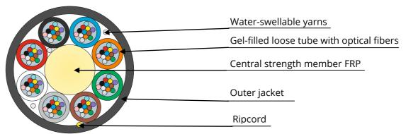
Cable consists of stranded core with central strength member (FRP), gel-filled loose tubes with optical fibers. Stranded core is fixed by water-swellable yarns. Outer jacket is made of polyamide PA12. Color of outer jacket is black. Ripcord is laid under the cable jacket.
