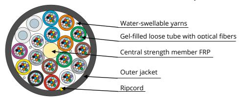
Cable consists of stranded core with central strength member (FRP) and two layers of gel-filled loose tubes with optical fibers and PBT fillers. Stranded core is fixed by water-swellable yarns. Outer jacket is made of polyamide PA12. Ripcord is laid under the cable jacket. Color of outer jacket is black.
