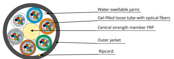
Cable consists of stranded core with central strength member (FRP), gel-filled loose tubes with optical fibers. Stranded core is fixed by water-swellable yarns. Outer jacket is made of polyamide PA12. Color of outer jacket is black. Ripcord is laid under the cable jacket.
