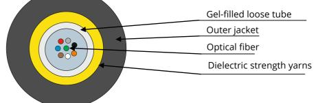
Cable consists of central loose tube (natural color) with optical fibers and water-blocking gel. Dielectric strength yarns are laid over loose tube. Outer jacket is made of PE. Color of outer jacket is black.
