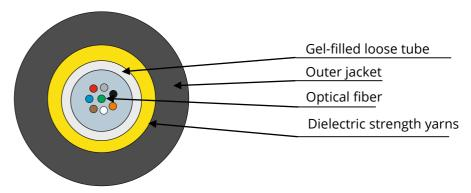
Cable consists of central loose tube (natural color) with optical fibers and water-blocking gel. Dielectric strength yarns are laid over loose tube. Outer jacket is made of PE. Color of outer jacket is black.
