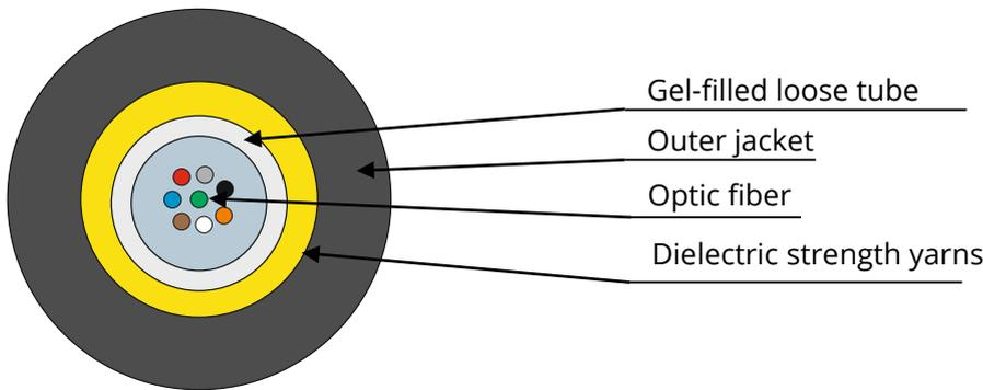
Cable consists of central loose tube (natural color) with optical fibers and water-blocking gel. Dielectric strength yarns are laid over loose tube. Outer jacket is made of PE. Color of outer jacket is black.
