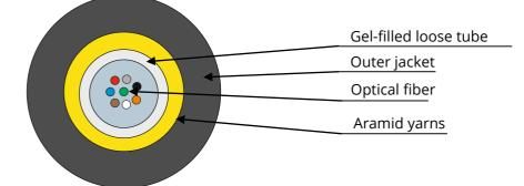
Cable consists of central loose tube (natural color) with optical fibers and water-blocking gel. Aramid yarns are laid over loose tube. Outer jacket is made of PE. Color of outer jacket is black.
